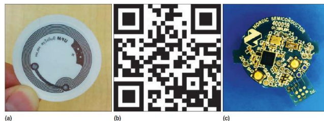
FIGURE 2. Various forms of electronic tags support the Physical Web (all about the size of a quarter): (a) a near-field communication (NFC) tag, (b) a quick response (QR) code, and (c) a Bluetooth low energy (BLE) tag. However, it is not clear which technology—each with its own affordances and problems—will become the primary IoT enabler.
